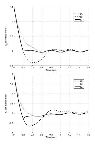
Figure 3: State estimation error  $\tilde{x}_3(t)$  and  $\tilde{x}_4(t)$  for each observer. (A) Dotted lines have been obtained by using the conservative PIO. (B) Dasehd lines have been obtained by using the oscillating PIO. (C) Solid lines have been obtained by using the ReO.
