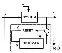
Figure 1: Reset observer applied to a LTI system.
