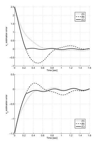
Figure 2: State estimation error  $\tilde{x}_1(t)$  and  $\tilde{x}_2(t)$  for each observer. (A) Dotted lines have been obtained by using the conservative PIO. (B) Dasehd lines have been obtained by using the oscillating PIO. (C) Solid lines have been obtained by using the ReO.
